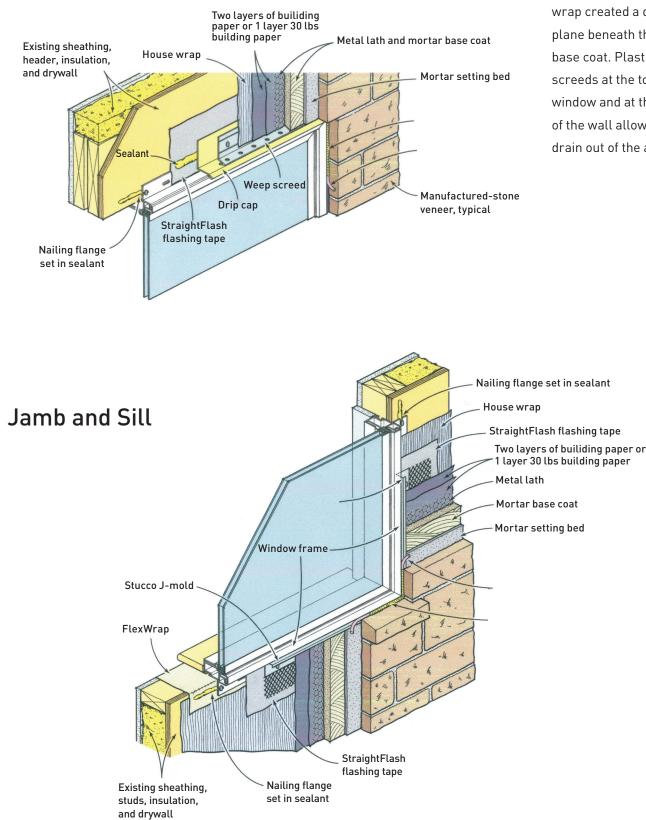
paper installed over house wrap created a drainage plane beneath the mortar base coat. Plastic weep screeds at the top of the window and at the base of the wall allow water to drain out of the assembly.
